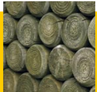
Palisades impregnated with Korasit ® CKF
